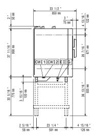
CWII Cold Water inlet 1 CWI2 Cold Water Inlet 2
